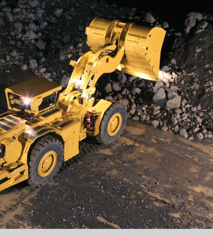
The R1300G underground loader is designed for high production, low cost-per-ton loading and tramming in underground mining applications. Compact design with agile performance, rugged construction and simplified maintenance ensures excellent productivity, long life and low operating costs.
